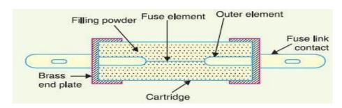
High voltage cartridge fuses are used upto 33 kV with breaking capacity of about 8700 A at that voltage. Rating of the order of 200 A at 6.6kV and 11 kV and 50 A at 33 kV are also available Types of Relays
