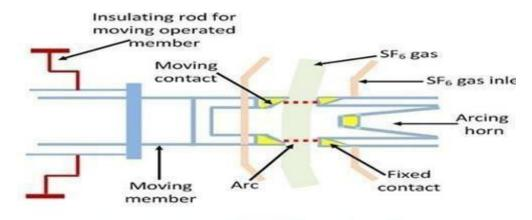
Interrupter Unit of SF6 Circuit Breaker
