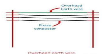
In case the resistance of electrical tower or ground is small, the lighting will be raised to very high voltage, which will cause a flash over from the tower to one or more phase conductors. Such a flashover is known as black flash over. Back flash over on the line can be minimized by reducing the tower footing resistance using driven rods and counterpoise where soil resistivity is high.
